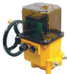
Model : UM-3-I Torque : 2070kgf-cm Operation Time/90° : 12/10sec 50/60Hz Mounting Flange : F07、F10、F12
