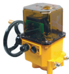
Model : UM-6-I Torque : 6100kgf-cm Operation Time/90° : 36/30sec 50/60Hz Mounting Flange : F07、F10、F12
