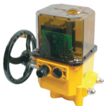
Model : UM-4-I Torque : 3800kgf-cm Operation Time/90° : 36/30sec 50/60Hz Mounting Flange : F07、F10、F12
