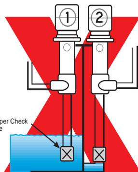
Check valves installed to maintain level. Not good to prime pumps
