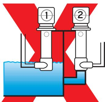
Solution level at impeller. No suction head available
