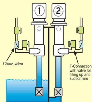
Solution level below impeller with priming tee. Check valve and throttling valve
