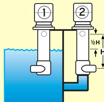
Liquid level halfway between discharge and weep hole
