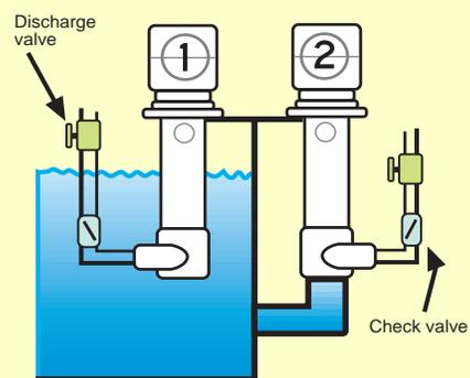
Solution level above impeller. Suction head available
