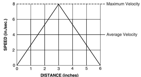
4. System peak flow can now be calculated using the peak velocity of the cylinder and the extend area. Peak flow in gpm =  $(V_m \times \text{area} \times 60)/231$  or  $(8 \times 3.14 \times 60)/231 = 6.53$  gpm peak flow.
